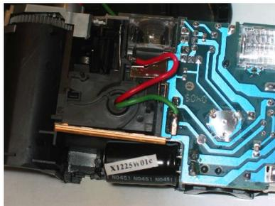
Thread both wires through the center hole and solder them as shown, red wire on the top, and green on the bottom. Do not reinstall the shutter and lens. Note the detail photos below: both wires are soldered to metal parts in the camera. The red wire is soldered to the little hook that held the shutter spring.
