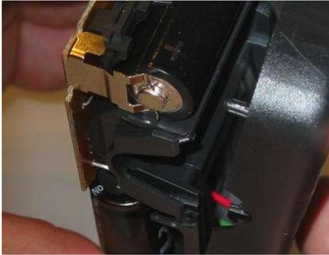
This detail shows that the “+” end of the battery goes into the “Y” shaped battery connector inside the camera.
