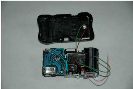
Install the 2.5mm connector into the hole in the plastic back.
