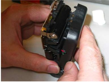
Snap the plastic front onto the camera **before** reinstalling the battery. Installing the battery will re-charge the Capacitor, so be careful! Note the polarity of the battery. If you put it in backwards, it permanently damages the circuit, and you will have to start over with new camera.
