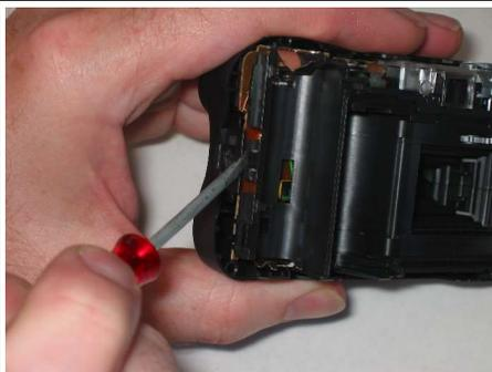
After you are **sure** that the capacitor has been discharged, gently pry off the latch that holds the plastic front.
