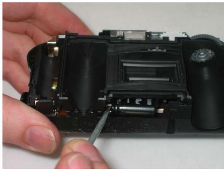
The flash capacitor might be charged up, even if the camera has never been used. The charged-up capacitor leads should be visible near the center at the bottom, when looking in through the back of the camera. Using the tip of a small, insulated, plastic-handled screwdriver, short the two capacitor leads together. You will probably see a flash and hear a loud pop.
