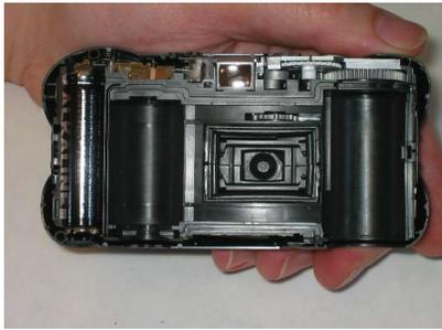
Remove the film and battery. The battery is shown on the left in this picture.
