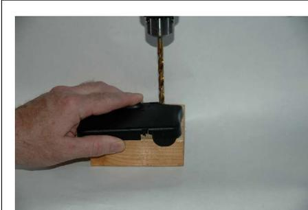
We mount our trigger connector on the plastic back, with the connector body taking the place of the film canister. Drill a 5/32" hole in the plastic back, as shown.
