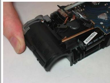
Beneath is the shutter, with a spring connected to it.
