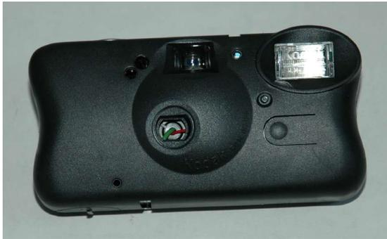
With the battery installed inside, snap the plastic front back onto the camera. Then snap the plastic back onto the camera, and the flash is complete. Congratulations, you are ready to take high speed photographs!
