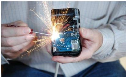
Here is a good photo of the spark that comes from discharging the capacitor. (But this photo is out of sequence, we haven't disassembled the camera this far yet.)
